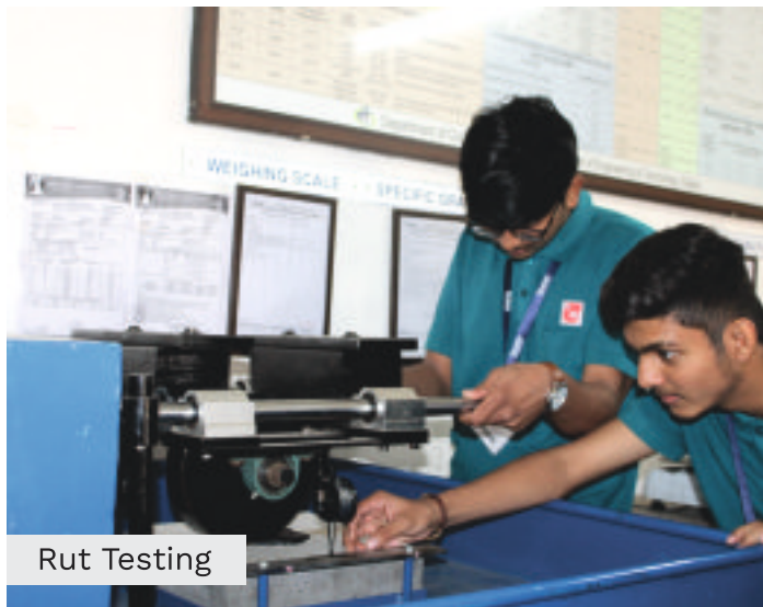
Bituminous Mix Designs
